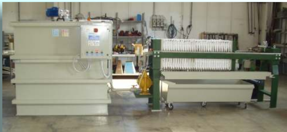
IMPIANTO DEPURAZIONE ACQUE MODELLO "CON FILTROPRESSA" PLANT TO PURIFY WATER - MODEL WITH FILTER-PRESS
